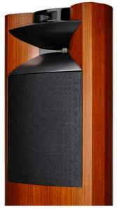
That curved front baffle provides the sidewalls for the main horn, while the top and bottom sections are made of precision-moulded Sonoglass. The supertweeter is also horn-loaded - in this case it sits behind a dedicated Sonoglass horn.
